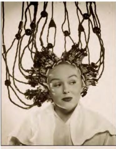
*Ed Note: These machines appears dangerous when I look at the bare electric wires that are exposed in the clips. Carol has told me that many women while undergoing “treatment” with this machine would lose some of their hair because the machine got too hot and burned the hair. The device many times resulted in a so called “Pocket Perm”. So called because when the victims hair got burned and the hairdresser removed the burned hair and quietly put the burned hair into her pocket. Nothing was said.*
